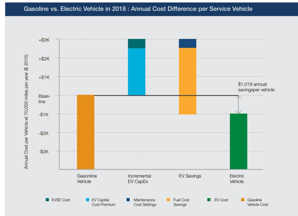
Figure 5. The relative economics of high-mileage EVs vs. ICEs shows that high-mileage EVs' will benefit from an approximately \$1,000 annual cost advantage in 2018. Source: RMI, Peak Car Ownership, 2016
