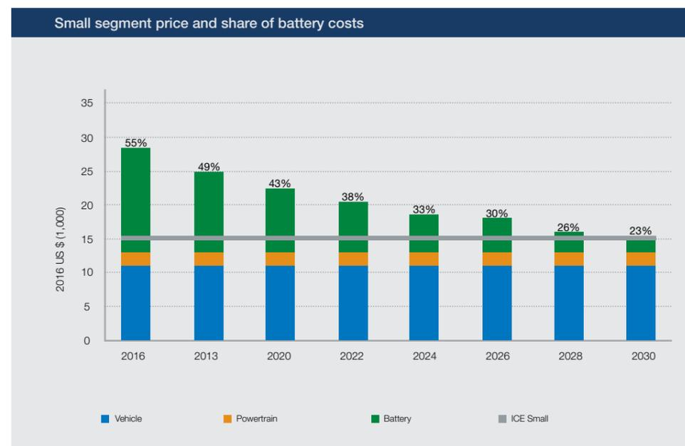
**Figure 8.** Batteries currently make up over half of the capital cost stack of EVs. While industry analysts expect batteries' share of and the total capital cost of EVs to come down over time, battery swapping can make some vehicle segments economic today. Source: Bloomberg New Energy Finance <sup>68</sup>
